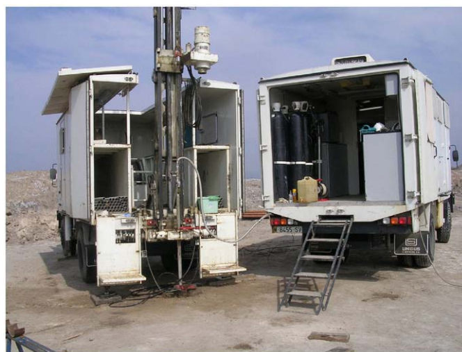
Fig. 3. Photograph of the Mobile Hydrogeological Unit operating in the field. On the left, one can see the descent vehicle and on the right the base vehicle.
