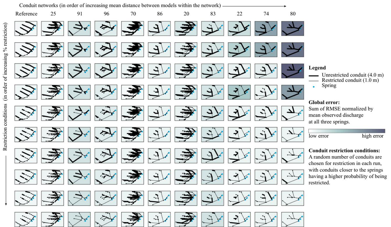
**Fig. 10** Model performance across ten different conduit networks in the subensemble, with ten different parameter sets (conduit restriction conditions) for each network. Each column represents a different network, sorted in order of increasing mean distance between models in that network (mean sum of squared differences, Eq. 2). Each row is made up of SWMM runs with different conduit diameter sets for that network,
