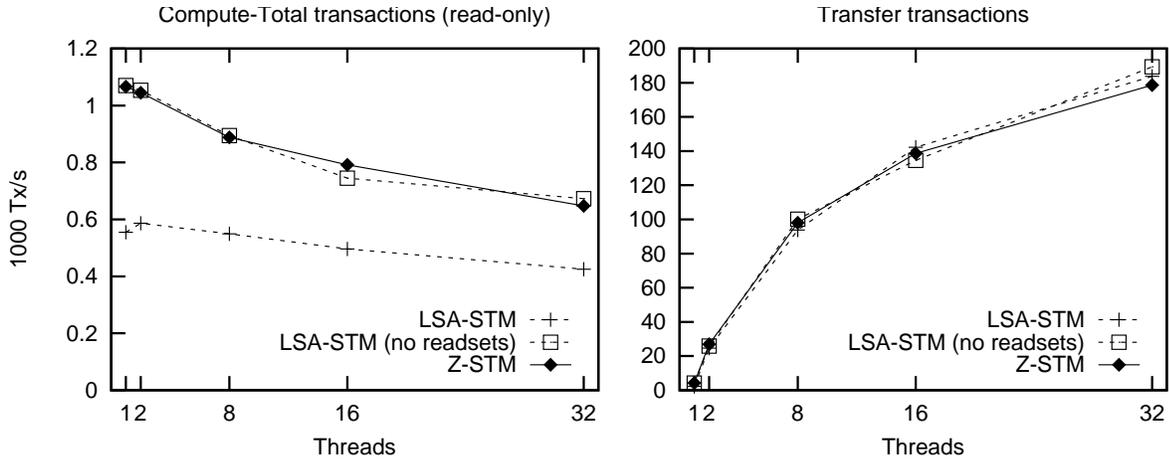
Figure 6: Throughput results for the Bank benchmark with read-only Compute-Total transactions.
