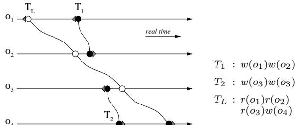
**Figure 1:** Linearizability schedules  $T_1$  before  $T_2$ , which forces long transaction  $T_L$  to abort (each transaction executes in a separate thread). Serializability would allow all three transactions to commit.
