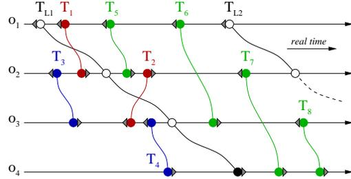
Figure 4: Long transactions have typically a higher chance of interfering with other transactions. Since the first committer wins, a commit by any of the short transactions  $T_5$  and  $T_6$  will result in the abort of  $T_{L1}$ .
