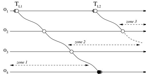
Figure 5: Long transactions partition short transactions into zones. Transactions in each zone are linearizable while the set of all transactions is only serializable.
