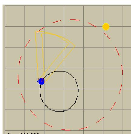
The robot aims to find the light source, which is placed in a rectangular area outside its closed neighborhood. The robot has two light sensors and can only sense the light if it is close enough to it. The robot acts based on the output of the
